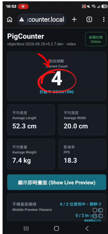
Figure 4-1: While counting — headcount and average length/width/weight update in real time
