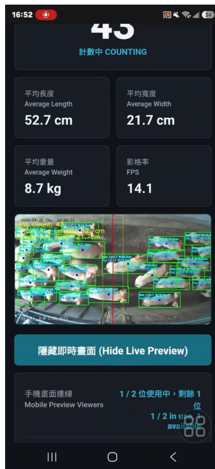
Figure 4-2: Live preview open, showing AI detection boxes, the counting reference line, and live overlay text
