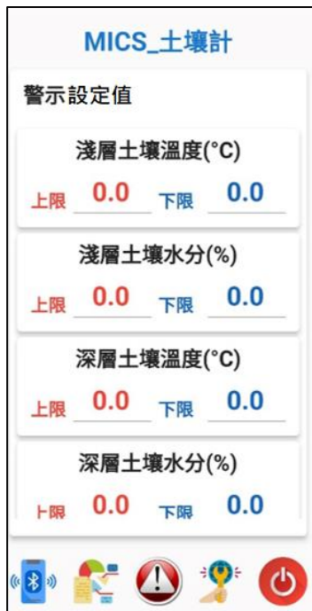
Step 13 soil temperature and moisture threshold value can be set
